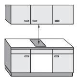
When two or more appliances are installed together below a cooker hood, e.g. a grill and an induction hob combiset, which have different safety distances given in the installation instructions, you should select the greater distance of the two.
